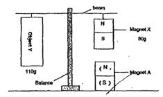
(b) As magnet X is light than object and needs to be pulled down to balance object Y and the magnet was attracted as their unlike poles were facing each other.
